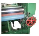
Bearing embedded continuous take-up mechanism
